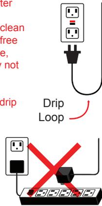
**CAUTION:** The heater must be fully submersed in water at all time. **MUST USE GFCI (Ground Fault Circuit Interrupter)** Do not plug into an extension cord/power strip.
