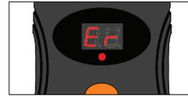
If the unit controllers LED reads "ER". The unit is over heated:
